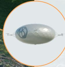
HS Airship is a **normal participant** of the **air traffic flow**, using autonomous but correctable flight planning, transponders, communication with the ATC, and sense-and-avoid functionality.
